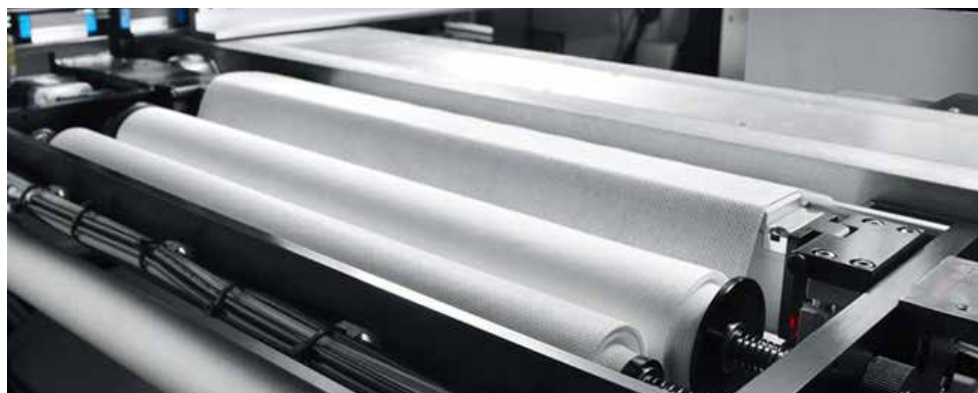
Programmable, Flexible stencil cleaning system: bottom side, wet, dry vacuum
