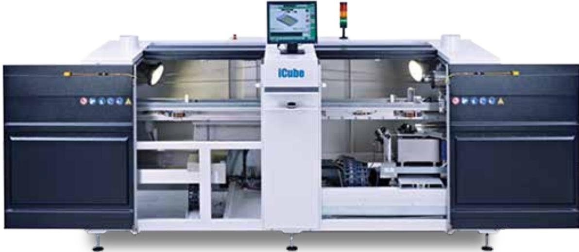
With the new iCube inline system, Absolute EMS can process three PCBs simultaneously: one PCB in the fluxer, one PCB in the preheat station, and one PCB in the soldering station, ensuring faster cycle times.
